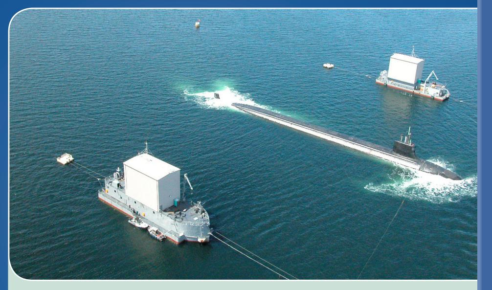
Submarines are critical assets used by the Navy to defend the United States and its interests, and the stealth of a submarine is of the utmost importance. SEAFAC ensures the highest level of stealth by measuring the precise level of sound emitted from a submarine, called an "acoustic signature."
