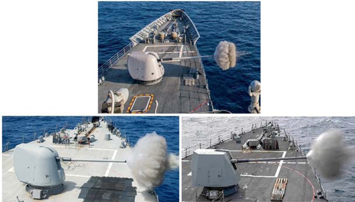
Figure 3.0-1: Gun Blast and Projectile from a MK 45 MOD 2 5 in./54 Caliber Navy Gun on a Cruiser (top), a MK 45 MOD 2 5-inch/54 Caliber Navy Gun on a Destroyer (bottom left), and a MK 45 MOD 4 5-inch/62 Caliber Navy Gun on a Destroyer (bottom right)
